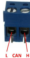
Figure 42: CAN0 Terminal Block
