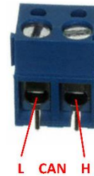
Figure 42: CAN0 Terminal Block
