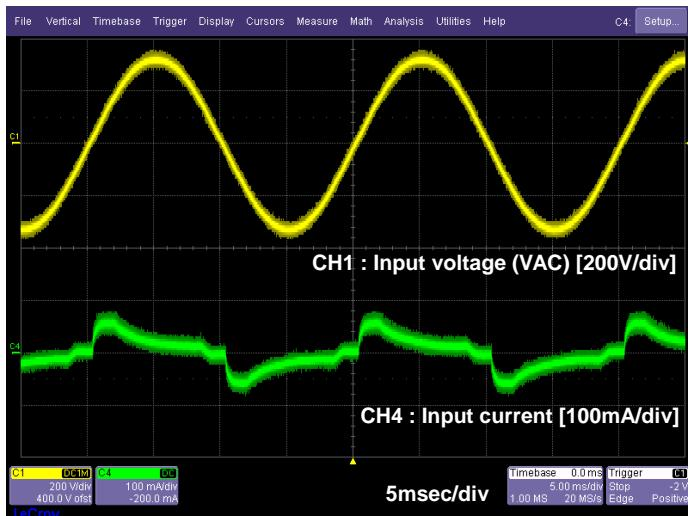
**Figure6.** Input waveform
