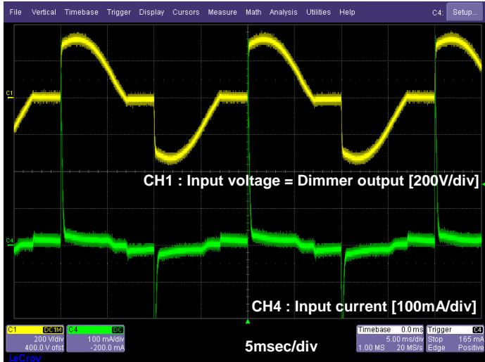
**Figure9.** Dimming operation waveform at
