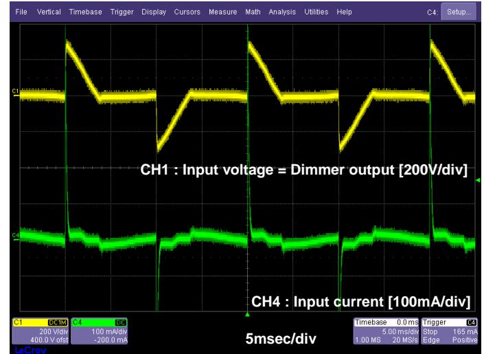
**Figure10.** Dimming operation waveform at
