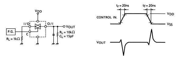
7. Total Harmonic Distortion, f<sub>max</sub> (I/O-O/I), Feedthrough (switch OFF)
