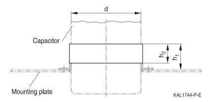
It is recommended to insert an additional insulating strip between capacitor and ring clip to avoid any risk of damage due to edges from the clip. The strip is included in delivery. For ordering code, see the following table. Attention must be paid to any relevant regulations (e.g. VDE, BSA or UL).
