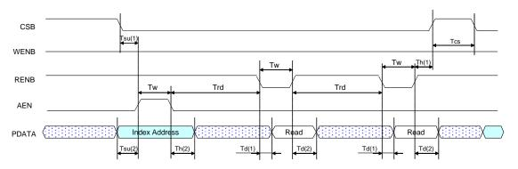
Fig 78 Read timing of parallel interface with auto index increment mode
