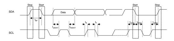
Fig 76. Serial Interface Timing Diagram
