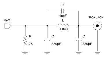
Fig 64 Example of reconstruction filter
