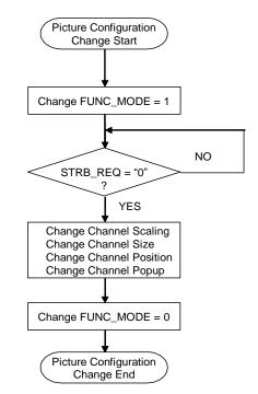
Fig 21 The sequence to change picture configuration
