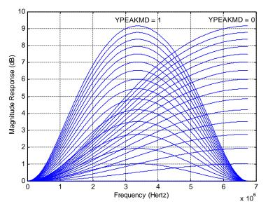
Fig 6 The frequency characteristic of luminance peaking filter
