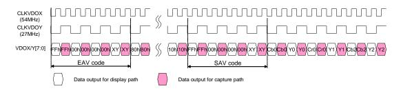
Fig 67 Timing diagram of dual output mode for 656 Interface
