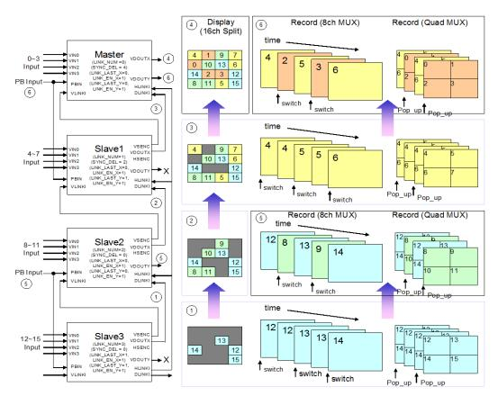
Fig 50 The cascade connection for 240 CIF/sec record mode
