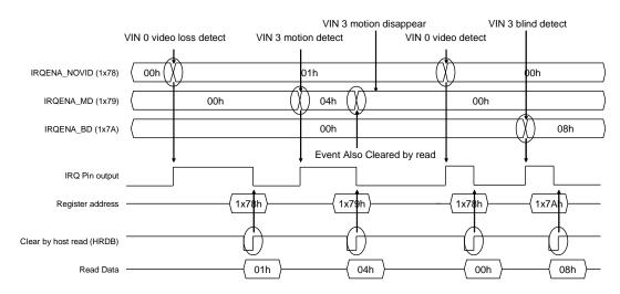
Fig 74 the illustration of Interrupt Sequence
