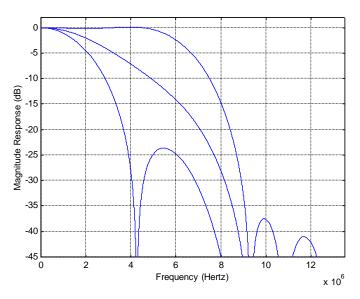
Fig 62 Characteristics of luminance filter
