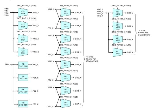
Fig 20 Channel input selection
