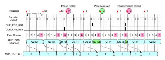
Fig 25 The illustration of QUE\_POS\_RST and QUE\_CNT\_RST
