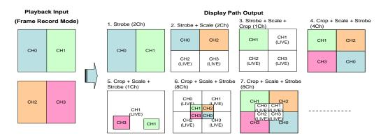
Fig 33 The examples of the playback function for frame record mode
