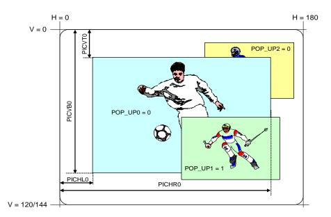
Fig 29 The channel position and priority in display path
