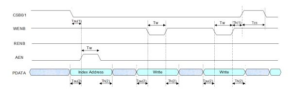
Fig 72 Write timing of parallel interface with auto index increment mode
