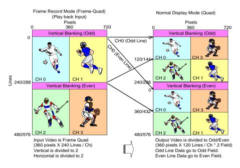
Fig 34 The conversion from frame record mode to normal display mode
