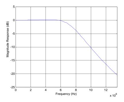
Fig 2. The frequency response of anti-aliasing filter
