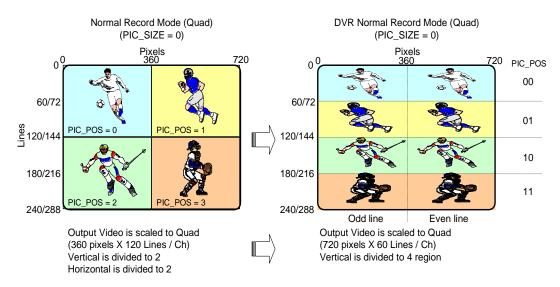
Fig 41 The channel position and size control for DVR normal record mode
