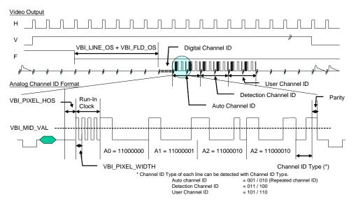
Fig 10 The related register for manual channel ID detection
