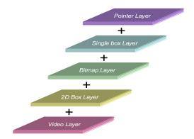
Fig 54 The overlay priority of OSD layer
