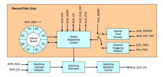
Fig 24 The structure of switching operation when QUE\_SIZE = 7
