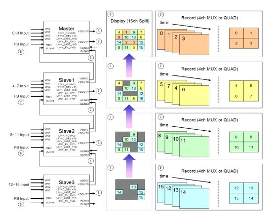
Fig 51 The cascade connection for 480 CIF/Sec record mode
