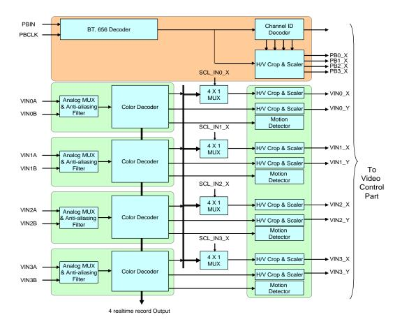
Fig 1 The structure of video input
