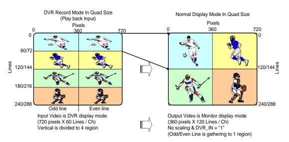
Fig 36 The conversion from DVR normal record mode to normal display mode
