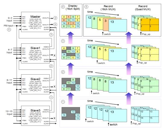
Fig 49 The cascade connection for 120 CIF/sec record mode
