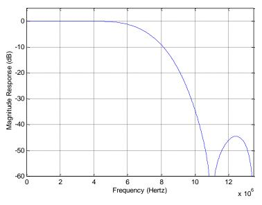
Fig 3 The frequency characteristic of the decimation Filter
