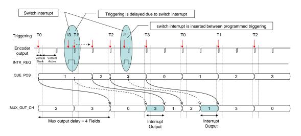
Fig 27 The interrupted switching sequence when QUE\_SIZE = 3, QUE\_PERIOD = 1
