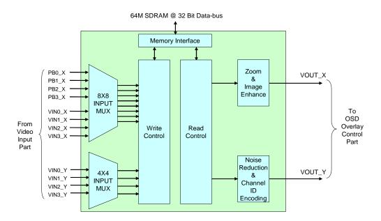
Fig 19 Block diagram of video controller
