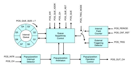
Fig 48 The structure of QUAD\_MUX switching operation when POS\_SIZE = 7
