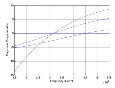
Fig 8 The frequency characteristics of IF-compensation filter
