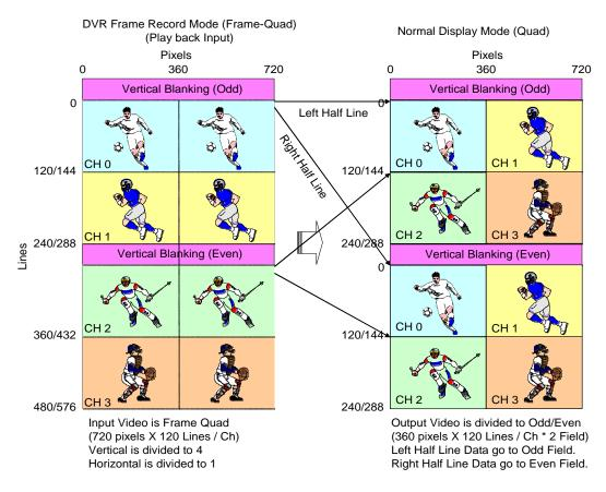
Fig 37 The conversion from DVR frame record mode to normal display mode
