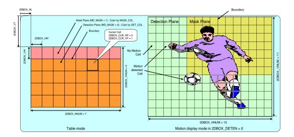
The following Fig 55 shows the 2D arrayed box of table mode and motion display mode.
