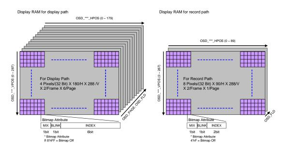
The following Fig 57 shows the structure of the display RAM in display and record path.
