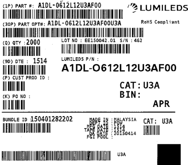
Figure 13. Example of a moisture barrier bag label.
