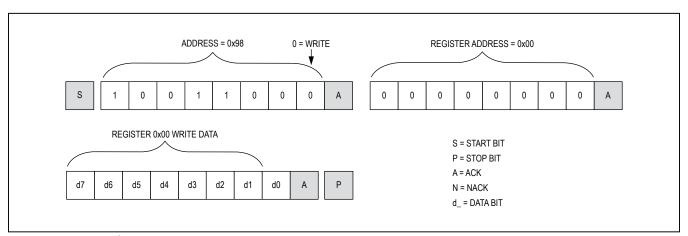
Figure 8. Format for I<sup>2</sup>C Write
