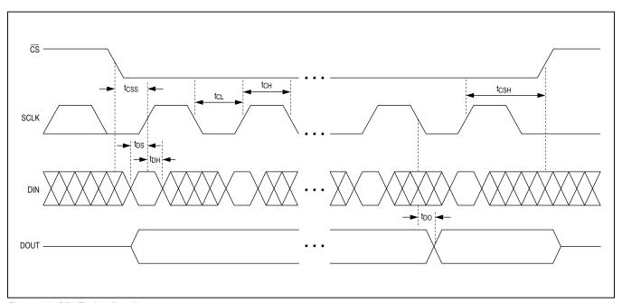
Figure 10. SPI Timing Details
