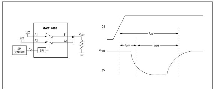
Figure 2. Turn-On/Turn-Off/Break-Before-Make
