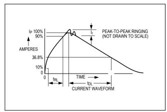
Figure 13. Human Body Current Waveform
