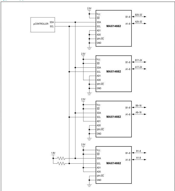
Figure 14. I<sup>2</sup>C 32 Switches
