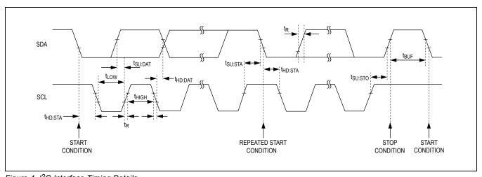
Figure 4. I<sup>2</sup>C Interface Timing Details
