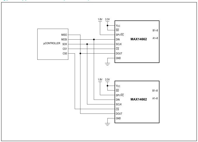
Figure 16. SPI Separate CS
