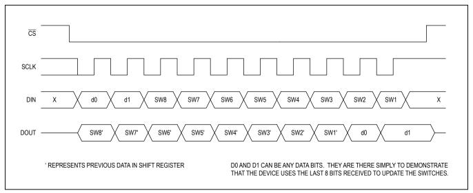
Figure 11. SPI Timing Diagram
