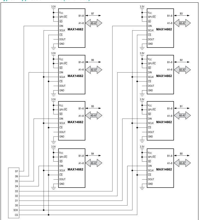
Figure 17. SPI Separate Data 8:8 crosspoint
