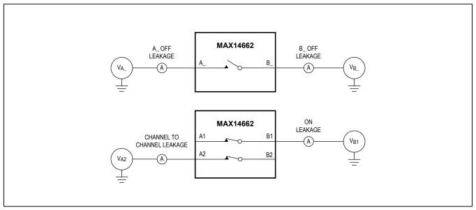
Figure 1. On-/Off-/Channel-to-Channel Leakage Current
