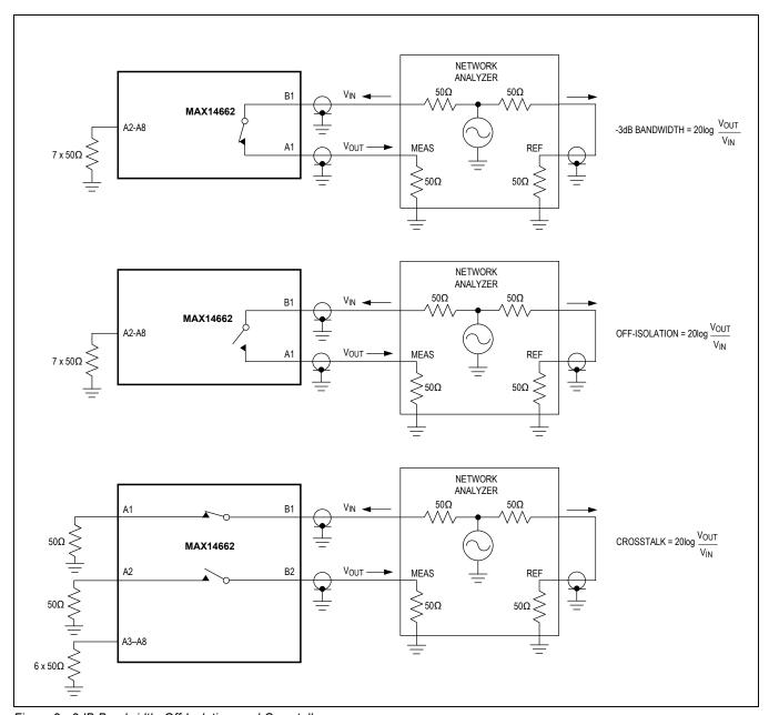
Figure 3. -3dB Bandwidth, Off-Isolation, and Crosstalk
