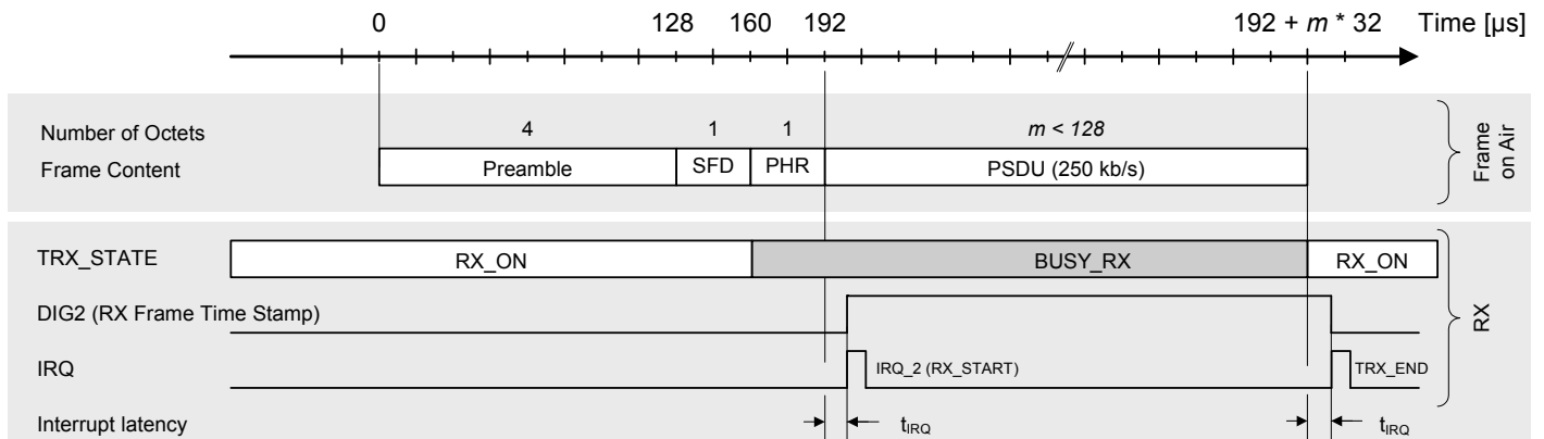
Figure 11-12. Timing of RX_START and DIG2 for RX Frame Time Stamping
