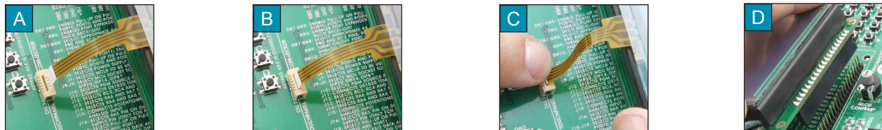
Figure 16-3: Connecting touch panel
