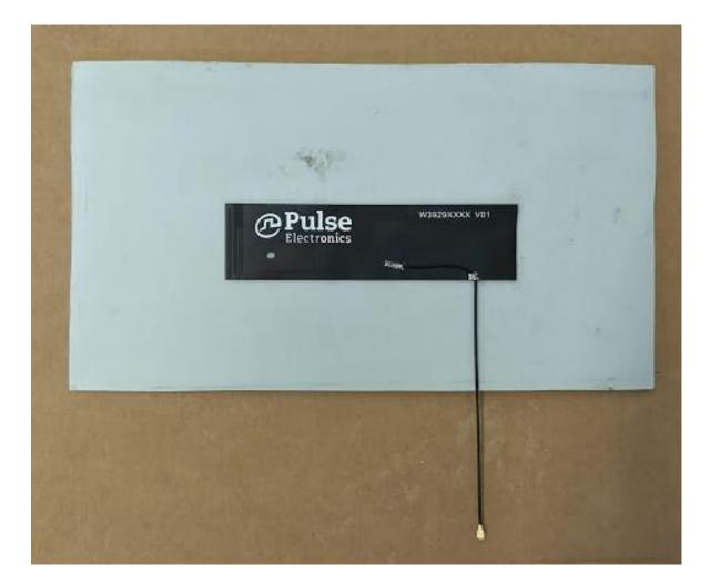
RF parameter testing is done when antenna is mounted on 2 mm thick plastic plate.
