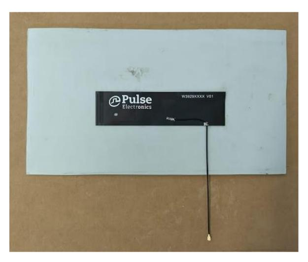
RF parameter testing is done when antenna is mounted on 2 mm thick plastic plate.
