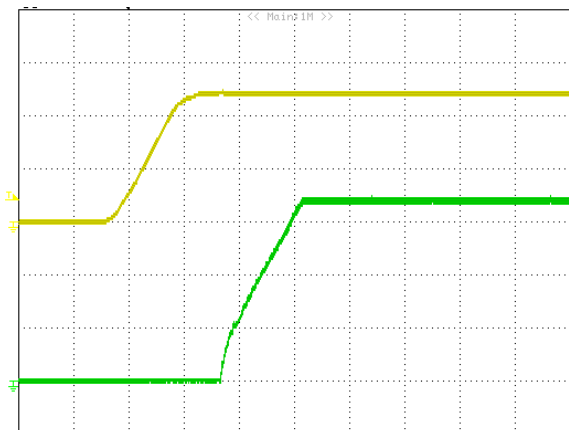
Figure 13: Turn on delay time at 12Vin, 1.8V/30A out. (Green : VOUT, 0.5V/div, Yellow: VIN, 5V/div. 1mS/div)
