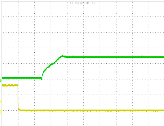
Figure 16: Turn on delay time at remote on 12Vin, 0.8V/30A out. (Green: VOUT, 0.5V/div, Yellow: ON/OFF, 2V/div, 1mS/div)
