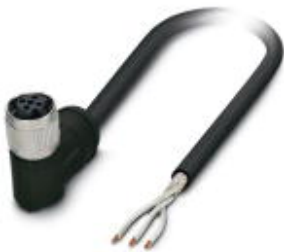
Sensor/Actuator cable, 3-position, PE-X halogen-free, black, shielded, free cable end, on Socket angled M12 SPEEDCON, A-coded, Cable length: 5 m, For railway applications
