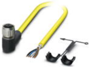
Sensor/Actuator cable, 5-position, PVC, yellow RAL 1021, shielded, free cable end, on Socket angled M12 SPEEDCON, A-coded, Cable length: 5 m
