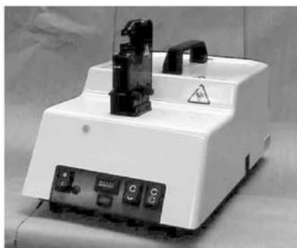
SDE Bench Terminator 1490076-2 (Customer Manual 409-10052)
