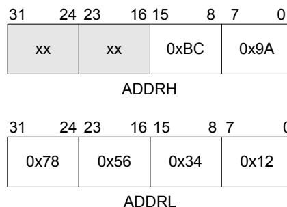
Figure 4.2 Example ADDRL, ADDRH Address Ordering
