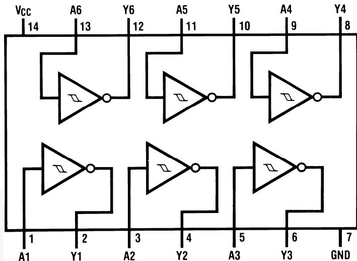
Figure 1. Pin Assignments
