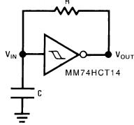
**Figure 3. Low Power Oscillator**
