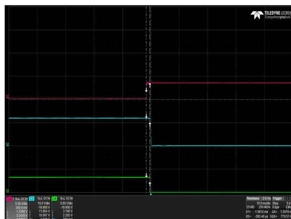
Figure 12: DS1600SPE-3 Turn Off Characteristic via PS_KILL_L Full Load: Io = 129.8A, Isb = 3.5A Ch 2: PS_KILL_L Ch 3: Vo Ch 4: Pwr_Good
