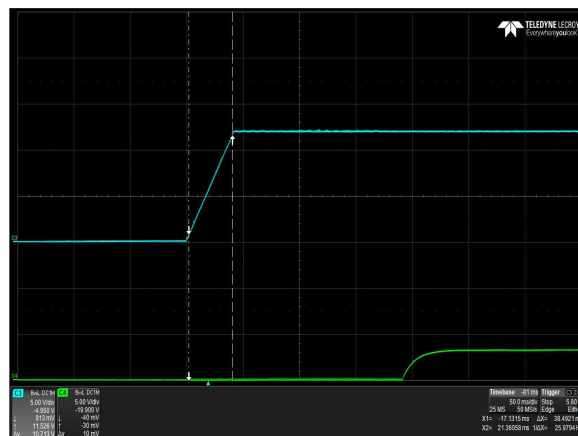
Figure 8: DS1600SPE-3 Output Voltage Startup – Vin = 180Vac Full Load: Io = 129.8A, Isb = 3.5A Ch 3: Vo Ch 4: Pwr_Good
