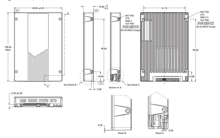
Note: 1. Length does not include 0.3 connector protrusion.
