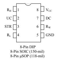
The DS1809 is available in standard 10 k $\Omega$ , 50 k $\Omega$ , and 100 k $\Omega$  resistor versions. The DS1809 is provided as an industrial temperature grade part only. Available packaging for the DS1809 include an 8-lead (300-mil) DIP an 8-lead (150-mil) SOIC, and an 8-lead (118-mil)  $\mu$ SOP.
