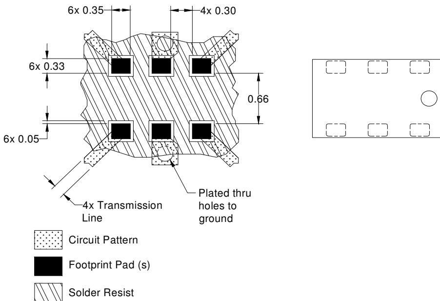
Dimensions are in Millimeters
