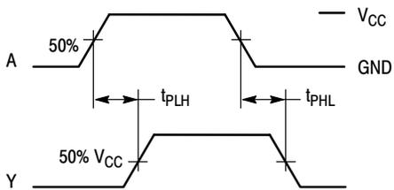
Figure 3. Switching Waveforms
