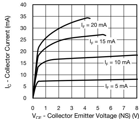
Fig. 4 - Collector Current vs. Collector Emitter Voltage (NS)
