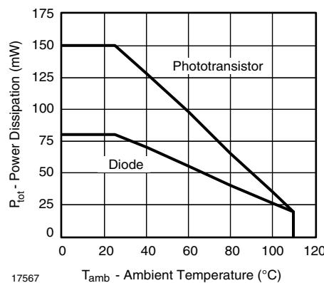
Fig. 1 - Permissible Power Dissipation vs. Temperature
