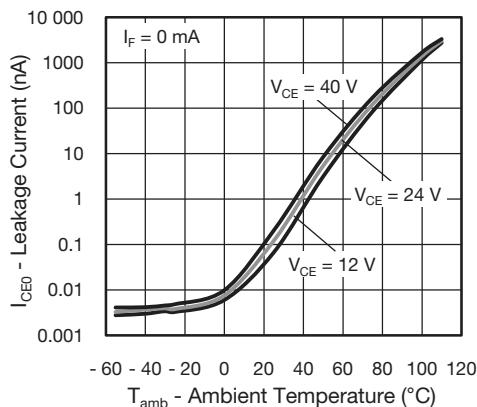
Fig. 5 - Leakage Current vs. Ambient Temperature
