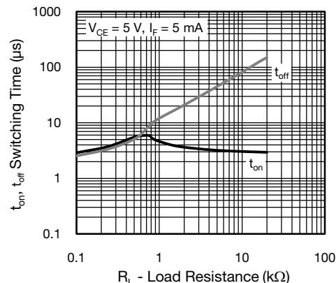
Fig. 13 - Switching Time vs. Load Resistance
