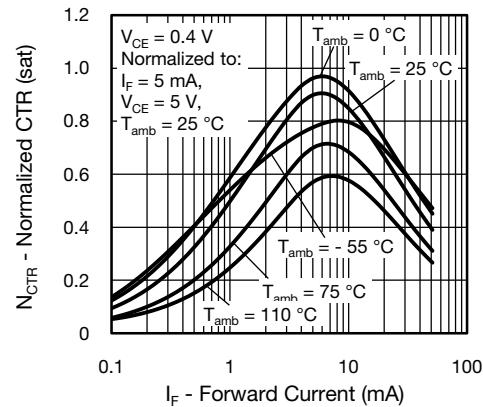
Fig. 9 - Normalized CTR (sat) vs. Forward Current
