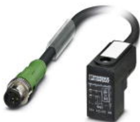
Sensor/actuator cable, 3-position, PUR halogen-free, yellow, Plug straight M12 SPEEDCON, A-coded, on Valve connector CI (9.4 mm), cable length: 1.8 m
