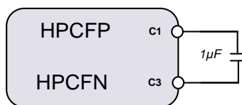
Figure 41: Charge Pump Flying Capacitor
