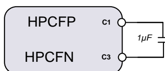
Figure 41: Charge Pump Flying Capacitor
