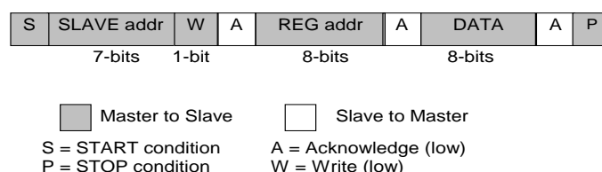
Figure 27: I 2 C Byte Write (SDA signal)
