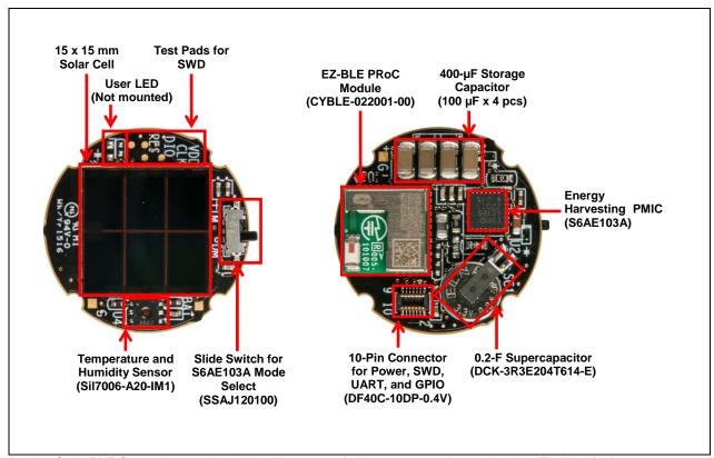
Note that the Solar BLE Sensor is not printed the silk screen of all components due to tiny size. To identify the components, refer to the assembly drawing shown in Figure 6-2.
