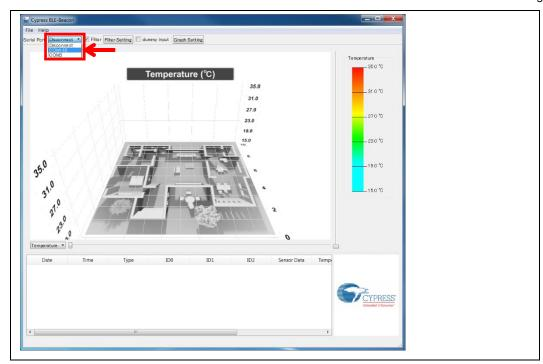
5. Find the **ID2** number (initial value is 0x0001) of the Solar BLE Sensor in the Cypress BLE-Beacon software. Refer to 3.3 Configuring Solar BLE Sensor to change the **ID2** number.
