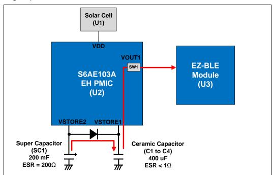
A few voltage drops will still occur, however, because VOUT is supplied using only a ceramic capacitor when there is no solar energy. The kit connects the 400- $\mu$ F capacitor to VSTORE1, and the energy of the BLE sensor transmission is about 200  $\mu$ J. If the VSTORE1 voltage is 1.9 V and it uses 200  $\mu$ J of energy, the voltage drop is about 0.28 V. Refer to the following equation.
