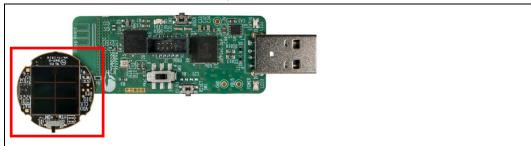
4. Plug the Debug Board with the Solar BLE Sensor into your computer's USB port. A supercapacitor (SC1) on the Solar BLE Sensor is charged when the Solar BLE Sensor is connected to the Debug Board via USB. Refer to Charging the Supercapacitor for detailed information.
