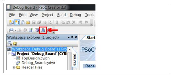
When PSoC Creator opens in debug mode, use the buttons on the toolbar for debugging. For more details on using the debug features, see the Cypress application note AN96841 – Getting Started with EZ-BLE Module or AN94020 – Getting Started with PRoC BLE.
