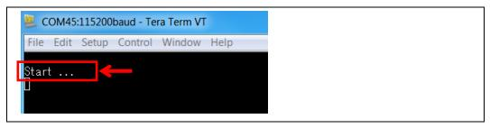
9. For example, this step will set the Major ID to "0x000a" (Hexadecimal) to receive another Solar BLE Sensor ID. On Tera Term, type *major 000A*. The Solar BLE Sensor responds with a confirmation message as follows. Refer to section 3.4 Serial Command List for a list of all kit commands.
