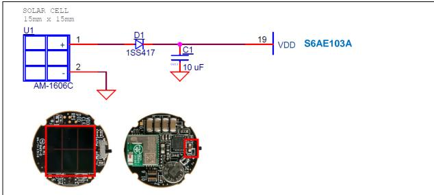
The following are the design specifications of the solar cell (AM-1606C).
