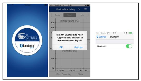
5. The BLE-Beacon app performs device discovery by default when the app is opened. Select the mode as **Graph** to display the sensor data.
