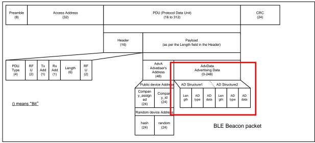
The following are the details of the BLE Beacon packet format for the kit.
