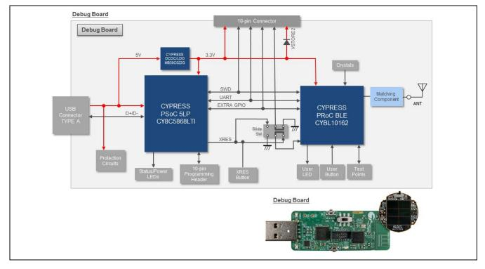
Figure 1-3. Block Diagram of Debug Board
