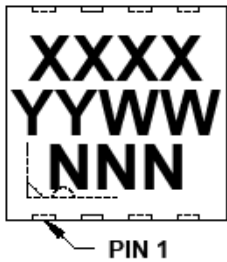
8-Lead DFN (3x3 mm)
