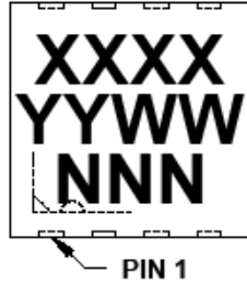
8-Lead DFN (3x3 mm)
