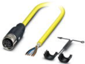
Sensor/Actuator cable, 5-position, PVC, yellow RAL 1021, shielded, free cable end, on Socket straight M12 SPEEDCON, A-coded, Cable length: 2 m
