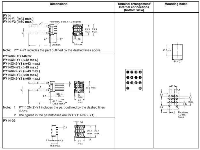
Note: 1. Use a panel with a thickness of 1 to 2 mm when mounting a Socket on it.
