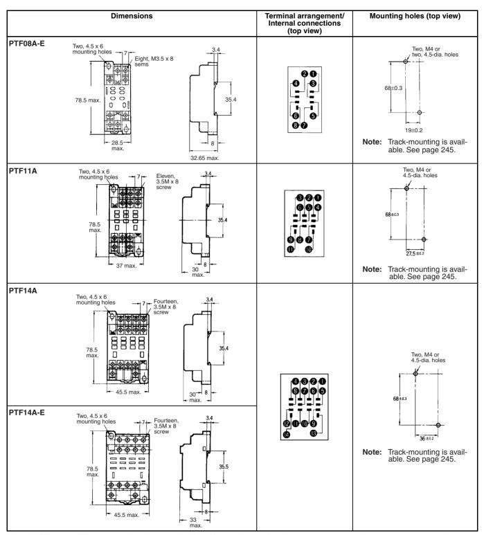
Note: If PTF08A and PT08 are used in combination with LY1 with a total current flow of 10 A minimum, terminals 1 and 2, 3 and 4, 5 and 6 respectively should be short-circuited.
