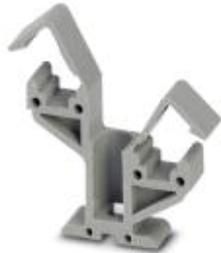
Double support, insulating material, optionally for use with 3 x 10 mm or 6 x 6 mm busbar, height in closed state: 39 mm
