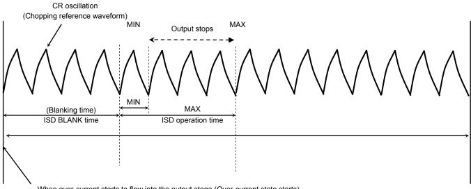
When over-current starts to flow into the output stage (Over-current state starts)
