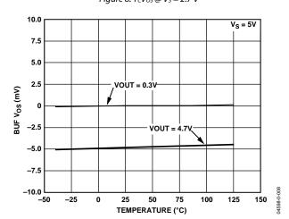
Figure 9. Output Buffer Offset vs. Temperature
