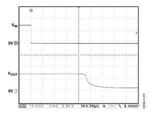
Figure 45. Positive Overload Recovery (Gain = 1280)
