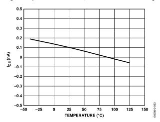
Figure 12. Input Offset Current vs. Temperature
