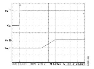
Figure 42. Negative Overload Recovery (Gain = 70)
