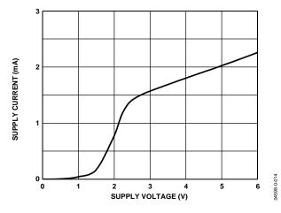
Figure 16. Supply Current (Isy) vs. Supply Voltage
