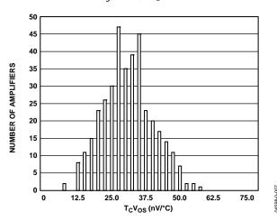
Figure 8.  $T_c V_{OS} @ V_S = 2.7 V$
