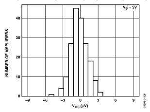
Figure 4. Input Offset Voltage Distribution
