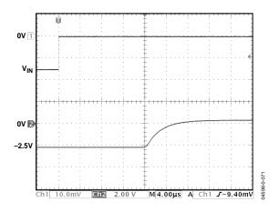
Figure 44. Negative Overload Recovery (Gain = 1280)
