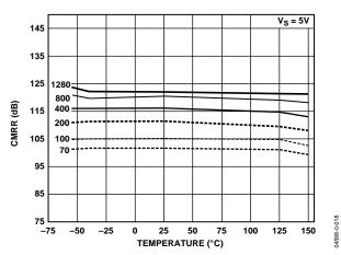
Figure 20. CMRR vs. Temperature at Different Gains
