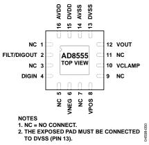
Figure 3. 16-Lead LFCSP (Not Drawn to Scale)
