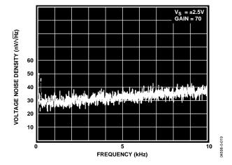
Figure 21. Input Voltage Noise Density vs. Frequency (0 Hz to 10 kHz)
