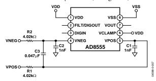
Figure 59. RFI Suppression Method
