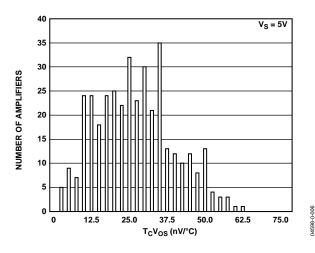
Figure 7.  $T_cV_{os} @ V_s = 5 V$
