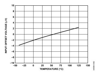
Figure 6. Input Offset Voltage vs. Temperature
