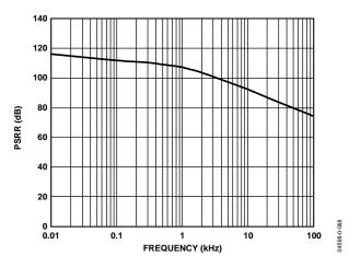
Figure 36. PSRR vs. Frequency
