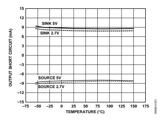
Figure 31. Output Short Circuit vs. Temperature
