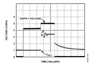
Figure 34. Power-On Response at −40°C
