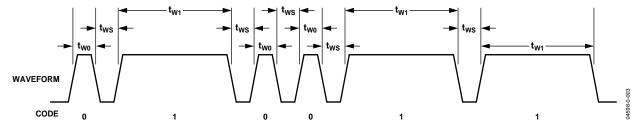
Figure 51. Timing Diagram for Code 010011
