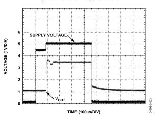
Figure 33. Power-On Response at 125°C
