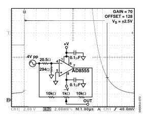
Figure 46. Settling Time 0.1%
