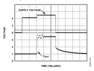
Figure 32. Power-On Response at 25°C
