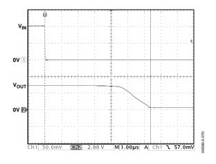
Figure 43. Positive Overload Recovery (Gain = 70)
