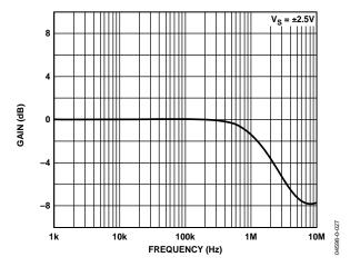
Figure 27. Output Buffer Gain vs. Frequency
