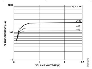
Figure 15. VCLAMP Current Over Temperature at  $V_S = 2.7$  vs. VCLAMP Voltage
