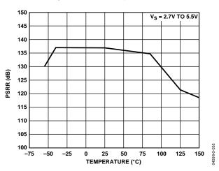
Figure 35. PSRR vs. Temperature
