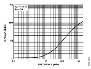
Figure 41. Output Impedance vs. Frequency
