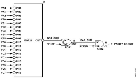
Figure 52. Functional Circuit of AD8555 Parity Check
