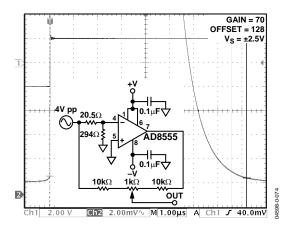
Figure 47. Settling Time 0.01%
