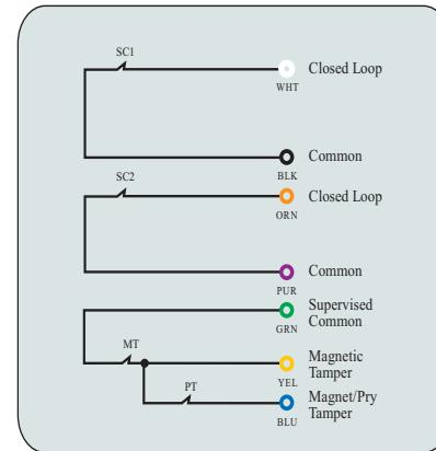
Dual alarm contacts both closed loop, with tamper circuit, closed loop.
