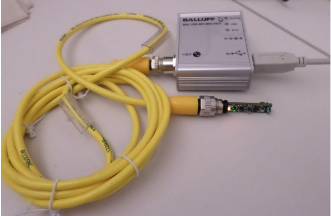
Figure 1. MAXREFDES27# Board Connected to a Balluff USB IO-Link Master
