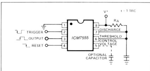
Figure 2. Maxim ICM7555 in a monostable operation.
