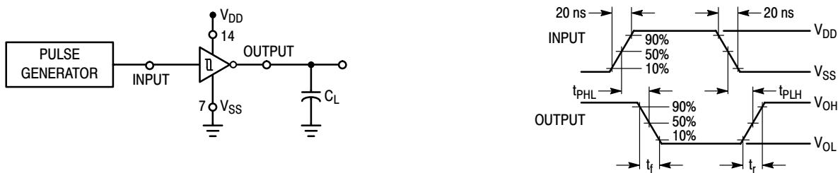
Figure 1. Switching Time Test Circuit and Waveforms
