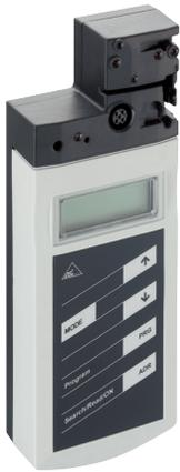
This AS-Interface Handheld controller serves to address the AS-Interface sensors, actuators and round cable modules. The mechanical connection is made by a mating M12 connector. AS-Interface flat cable modules are connected using the addressing adaptor type 0913 ATL 002/0.35 M. With this addressing equipment, all types of AS-Interface modules (including equipment with ASInterface Version 2.1) can be addressed.
