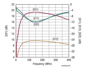
Figure 3. Demo Board S-Parameters
