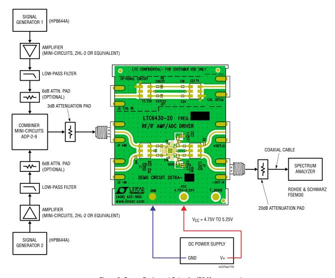
Figure 2. Proper Equipment Setup for IP3 Measurement
