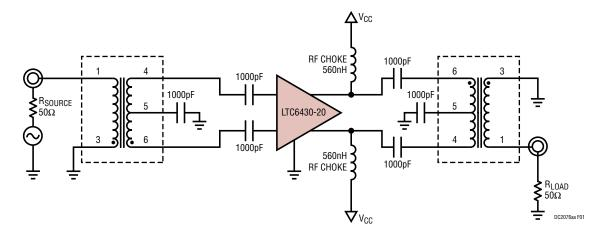
Figure 1. DC2076A-A Simplified Schematic
