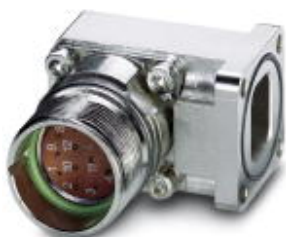
Device connector, front mounting, angled fixed, Screw locking, M23, number of positions: 17, type of contact: Socket, Crimp connection, Axial O-ring, 4x Ø 3.2, shielded: yes, flange dimensions: 26 mm x 26 mm
