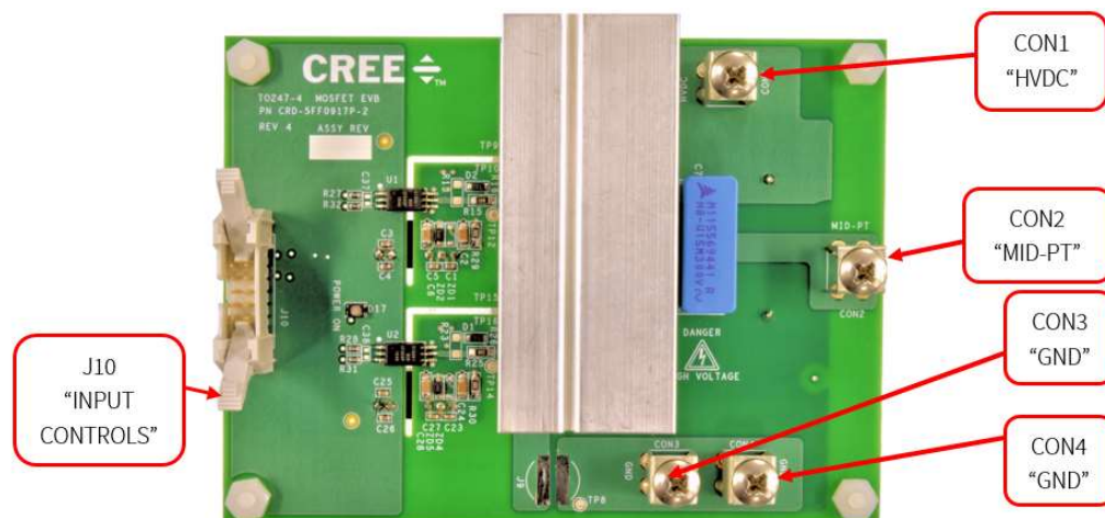
Figure 9. Top view of Cree's KIT8020-CRD-5FF0917P-2 evaluation board showing locations of various connectors
