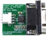
The RSLink2 converts between PIC UART signals and RS-232 required to communicate with a standard PC COM port. On the PIC side it connects to ground, power, and the UART receive and transmit lines. The RSLink2 supports power supply levels from 3.0 to 5.5 volts. The RS-232 interface is via a female DB-9 connector. It can be connected to a standard PC COM port with a straight through extension cable.
