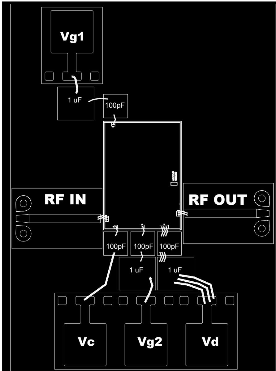
**To ensure low frequency stability, use 1uF surface mount (not leaded) capacitors (on the Vd, Vg1, and Vg2 nodes) that are located close to the MMIC. Contact TriQuint Semiconductor Applications Engineering for more details.**
