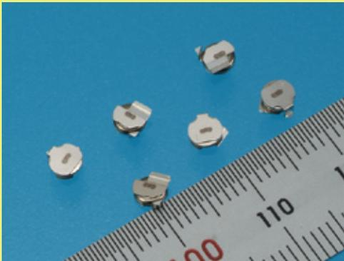
XH311HG is a coin type capacitor (D: 3.8mm / H: 1.1mm), with a unique quality of large current discharge, ranging from 3.3V to 0V. It is Pb-free reflowable with a high temperature heat resistance (Peak temperature of 260°C).
