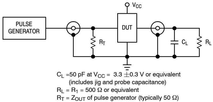
**Figure 4. Test Circuit**
