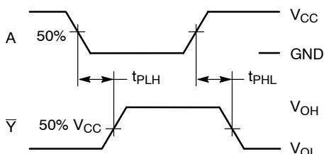
**Figure 3. Switching Waveforms**
