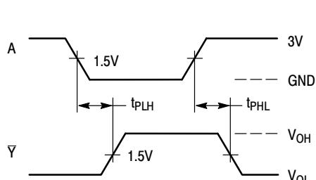
Figure 3. Switching Waveforms
