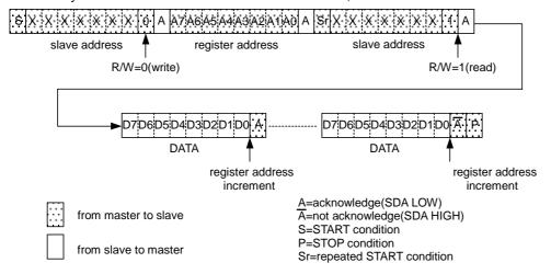
※ As for reading protocol and multiple reading protocols, please do Ā(not acknowledge) after doing the final reading operation. It stops with read when ending by A (acknowledge), and SDA stops in the state of Low when the reading data of that time is 0. However, this state returns usually when SCL is moved, data is read, and Ā (not acknowledge) is done.
