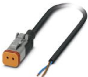
Sensor/Actuator cable, 2-position, PUR halogen-free, black-gray RAL 7021, free cable end, on Socket straight DEUTSCH DT06-2S Clip locking, with 1 LED, Cable length: 10 m
