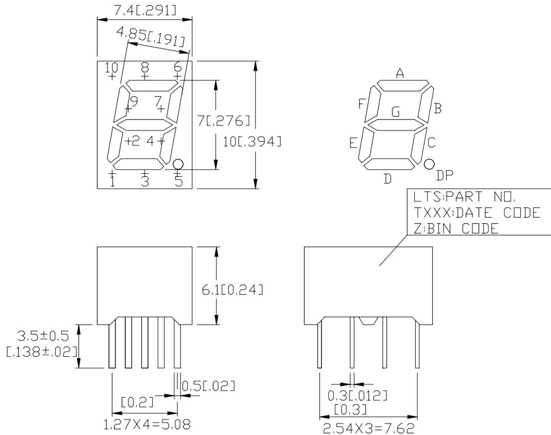
NOTES: All dimensions are in millimeters. Tolerance is ± 0.25 mm (0.01") unless otherwise noted.
