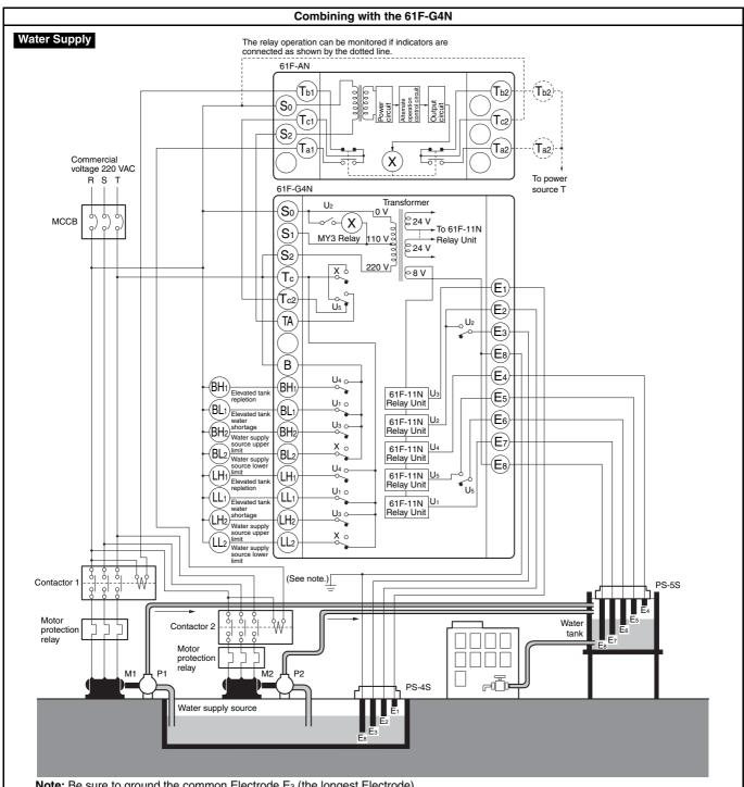
Note: Be sure to ground the common Electrode E<sub>3</sub> (the longest Electrode).
